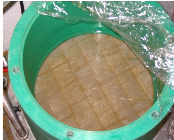
Figure 5..Gonflement sans contrainte (Photo CEMAGREF)
